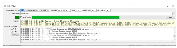
DIPCap is a replacement for RCAPTURE. RCAPTURE fails after a few days or weeks and only supports TCPIP 'Client' connections, DIPCap is very robust and will run forever. It has better logging and also supports TCPIP 'Server' connections.
