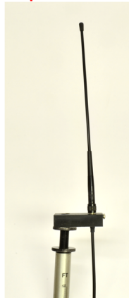
Figure 8 Raising the UHF antenna for additional range.
