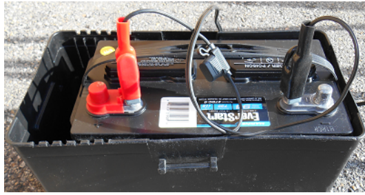
Figure 12 Alligator-clip connections won't support full output power!
