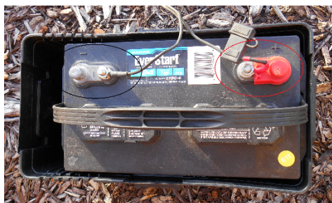
Figure 11 check the polarity of the connections to the battery before use.
