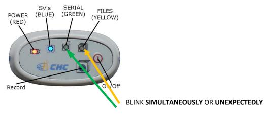
The head is 'locked up' if the ON/OFF button does not work.
