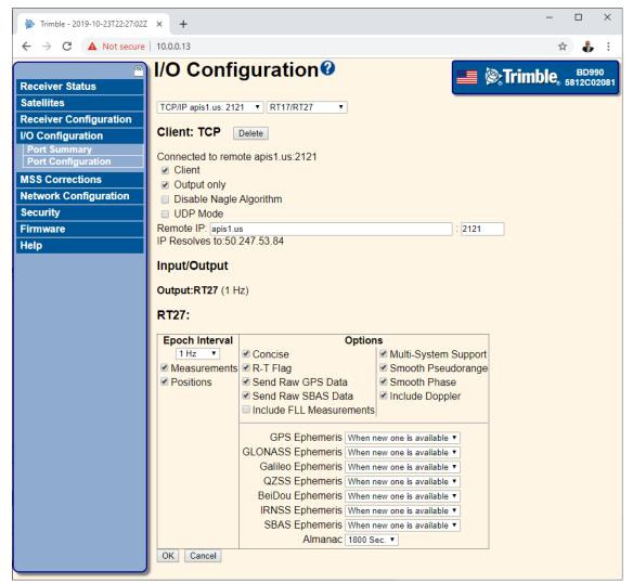
DO NOT check the 'Include FLL Measurement' checkbox, as TEQC is used to decode streams and FLL won't work. When configured to a matching port at the iGage stream server, hourly and daily files will be collected and archived.
