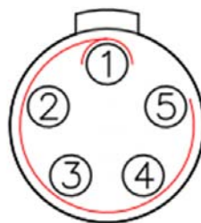
Figure 7 HJ394 C Port Welding Surface View
