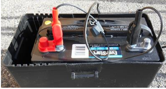
Figure 11 Alligator-clip connections won't support full output power!
