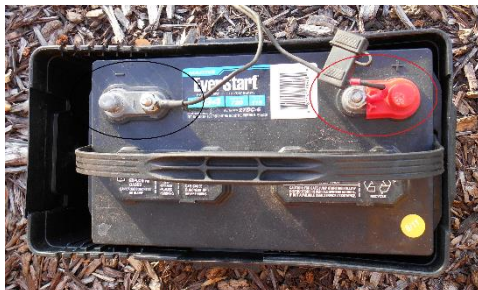
Figure 10 check the polarity of the connections to the battery before use.
