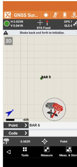
A translucent tilt indicator will be displayed on the map bottom. As the IMU initializes several prompts are shown. The symbol above requests that you need to rock the receiver back-and-forth on a point.
