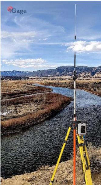
Works as a remote repeater or cable connected high power radio.
