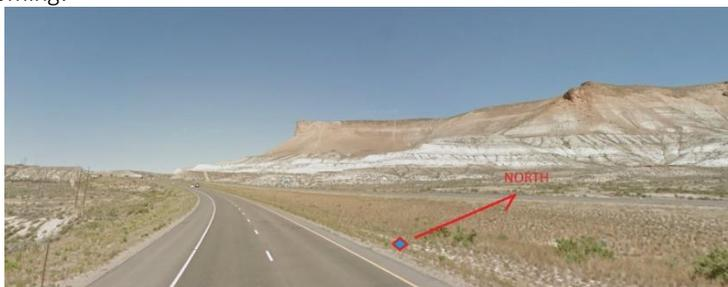
It has fantastic views in all directions, unfortunately a semi-truck drives by every 20-seconds and completely obscures a receiver's view of the southern sky. This forces the receiver (and OPUS) to lose lock. This is a **BAD** location and will greatly increase the RMS error estimates and drop the percentage of observations used.
