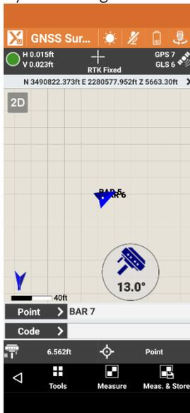
When this icon is shown, the tilt compensation is active and you can store a measurement.
