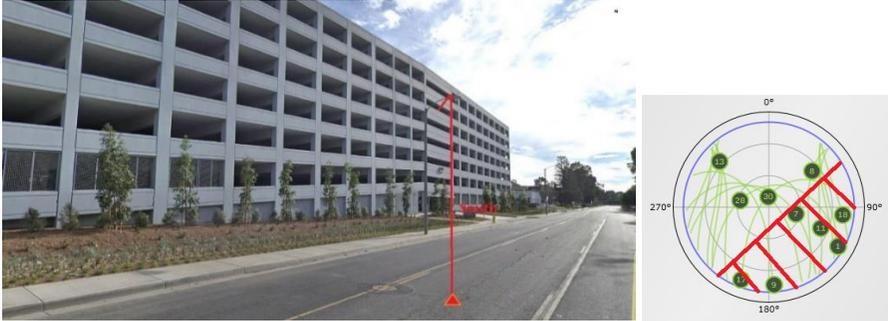
This is a **bad** location because the structure completely blocks the antenna's view to the South and East.
