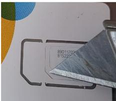
Use a knife blade to extract the correct nano sized card, the smallest punch out.
