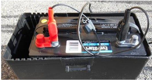
Figure 11 Alligator-clip connections won't support full output power!
