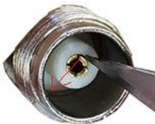
Bending the center contacts in towards the center.
