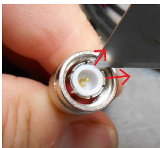
Bending out the ground contacts on the antenna connector.
