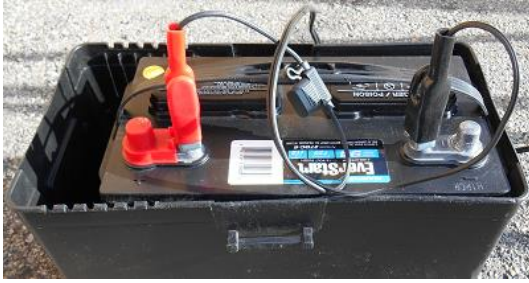
Figure 11 Alligator-clip connections won't support full output power!
