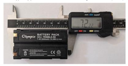
A battery is too long if you have to push the battery into the battery slot with high force in order to have the retaining clip secure the battery end.
