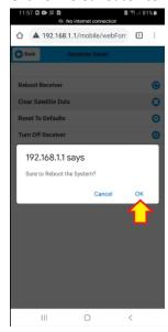
Wait for receiver to reboot. After it reboots, if it does not track SV's then turn the power off, wait 30 seconds and turn the power back on.
