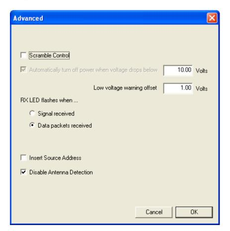
Uncheck Scramble Control. Typically we uncheck 'Disable Antenna Detection'.
