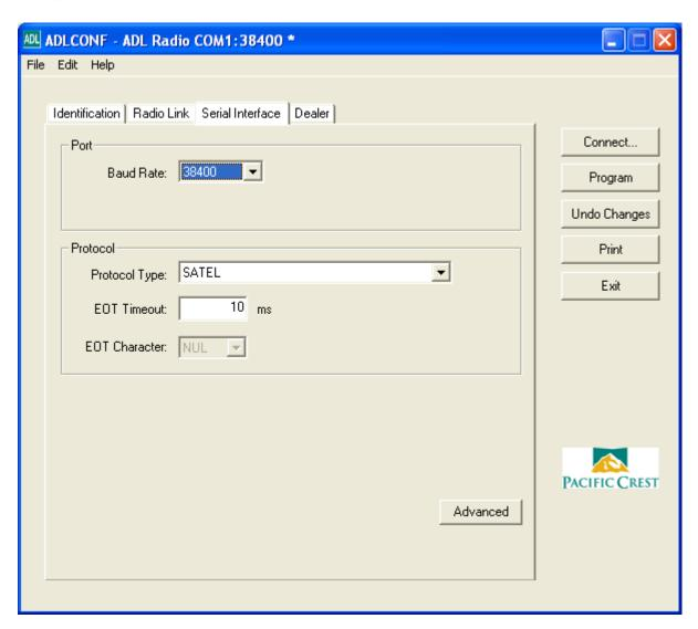
The baud rate above is the baud rate of the serial cable.
