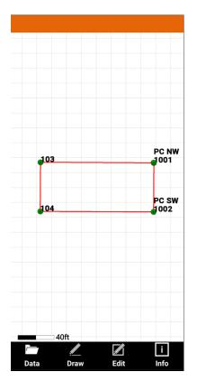
Points 101 and 102 are directly underneath 1002 and 1001 and the labels are not visible. You can verify this in the point list because the Northing and Eastings for the point pairs 101-1002 and 102-1001 are exactly the same.
