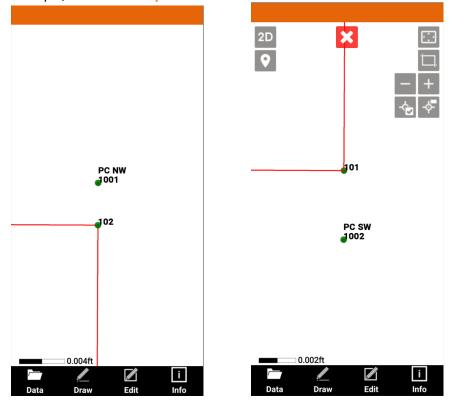
The resulting transformed distance from 102 to 1001 is 0.004 feet. The distance from 101 to 1002 is 0.004 feet.
