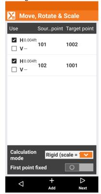
If First point fixed is OFF, then the result will balance the distance difference between the points. In other words, the resulting distance from 101 to 1002 will exactly equal the distance from 102 to 1001.
