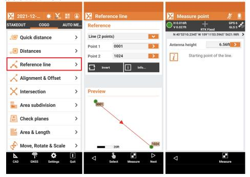
Click on Reference line, then click on Measure. This will allow you to set the starting point 1 of the line, click Measure again to set the Starting point at the current random point 25.00 feet from the target.
