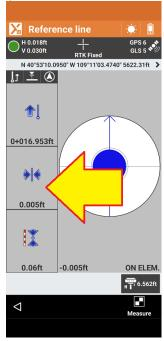
Move as close to the tree canopy as the rover will go, then move left/right to minimize the distance to line (0.005' above.)
