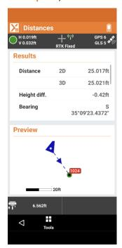
Move towards/away from the target point until the live 2D Distance Results is 25.00 feet with the rod leveled, drop your bi-pod feet to hold this position, exactly 25 feet from the target.
