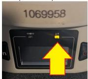
should be blinking once per second. Typically, amber is FLOAT, green is FIXED.
