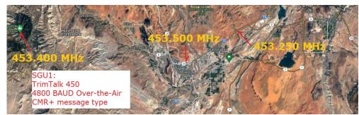
Correction Protocol Radio Protocol Over the air baud rate West (Utah Hill) Main (center of town) East (Washington City)
