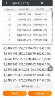
And the **NE Switch** Ne Switch button automates quickly exchanging the Northing and Easting order.
