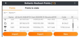
The list can be sorted ascending or descending by Name, Northing, Easting, Elevation, Code, Creation and Modified time by clicking on the column heading sort buttons:  $\triangle$ ,  $\triangleright$ .
