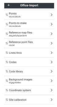
2.In the Import function, the imported data types can be sorted. Users can drag the commonly used ones to the front.
