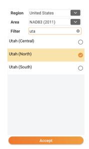
Set Region = United States, Area = NAD83 (2011) or another suitable region, type in a Filter, check the desired coordinate system and finally click Accept
