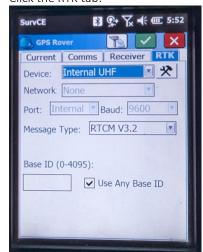
If you choose to change the Internal UHF settings by clicking the hammer wrench button, the radio setup process may fail.
