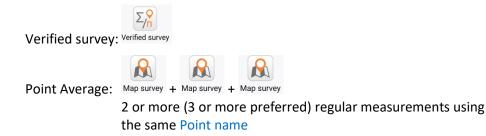
Since the Verified survey method forces a complete receiver initialization between groups, and allows for subsequently adding additional groups, it is the preferred measurement type for least squares analysis.
