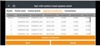
to view the computed adjustments to the group averages which best fit the measurement network. Usually, the suggested deltas will inconsequential when the underlying accuracy of GNSS measurements are considered.
