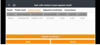
to view the Base **Control points** with the standard errors.
