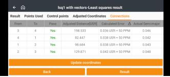
to see which parcel vectors passed the tolerances, the best-fit adjusted vector lengths, the calculated measurement error in PPM excess, the actual semi-major error which represents the greatest horizontal error at a station, the allowable semi-major error computed by the vector length \* PPM + tolerance and the ratio. Ratios less than 1 represent overly qualified vectors while ratios higher than 1 indicate a failing measurement.
