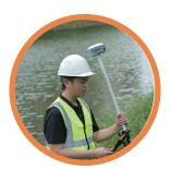
200 Hz AUTO-IMU eliminates manual initialization, Automatic pole tilt compensation,3 cm accuracy over a 60° tilt range, Saves up to 30% of time.
